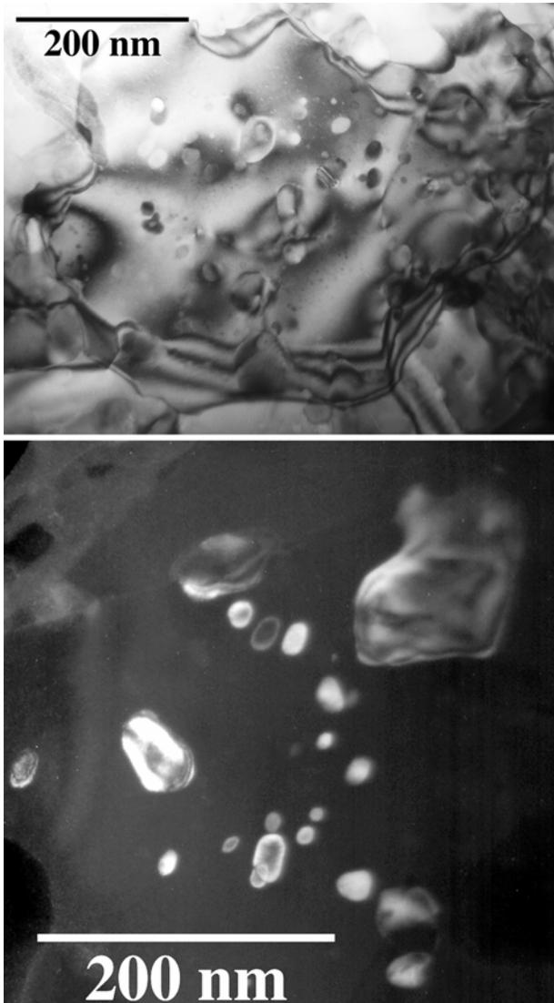
Fig.10: TEM a) bright and b) dark field views of Sn-Cu deposit approximately 24 h after electroplating.  $\text{Cu}_6\text{Sn}_5$  intermetallic particles were identified by SAD in the interior of the Sn grains and on the grain boundaries. The dark field images show that the internal particles share a common orientation.
